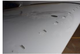
6kts. The airplane still breaks straight ahead in the stall but at a higher angle of attack, and is more controllable in slow flight. Vortex generator kits are manufactured for GA aircraft by Micro Aerodynamics
