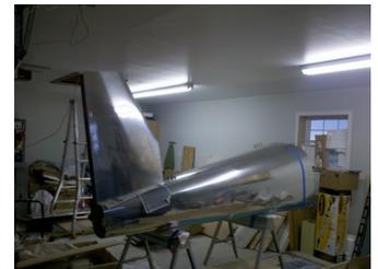
At the present time, I have completed the tail cone, the vertical stabilizer and rudder, and the horizontal stabilizer. That took about 125 hours. I started the wing kit last week, and it appears to be coming together faster.
